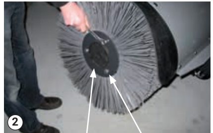
2 Disassembling the flange Bolt
