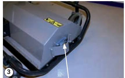
Lubricate the bearing on the right-hand side
