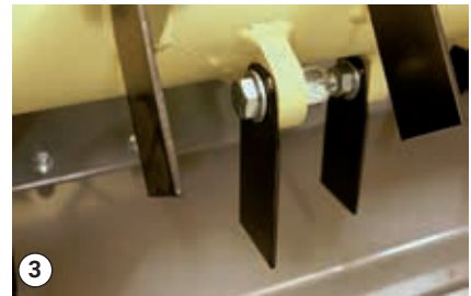
Vertical blades fitted individually
