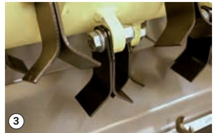
The flails are fitted together
