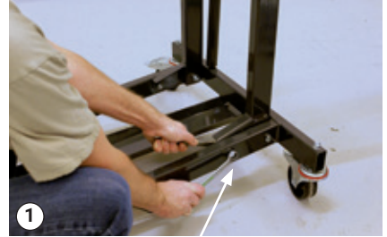
2 bolts on the tank frame
