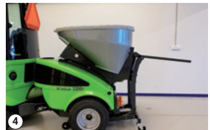
Mounting the salt and sand spreader
