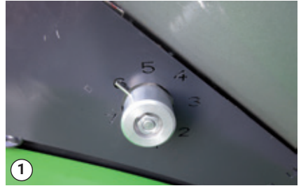
Adjusting the spread width
