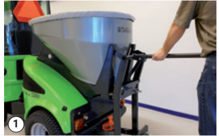
Salt and sand spreader being lowered onto the machine
