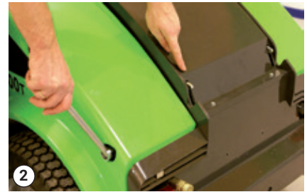
Locking lever – unlocked
