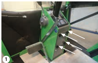
Sikringer i rattpanelet
