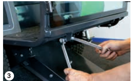
Bolts under base plate
