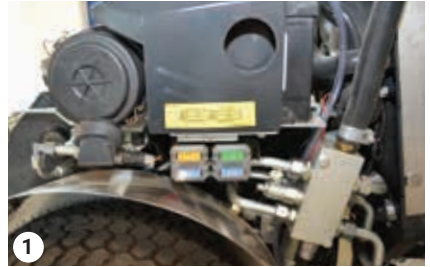
① 60 A JF15 generator - 60 A JF1 supply fuse box 20 A JF2 emergency line - 30 A JF3 engine power
