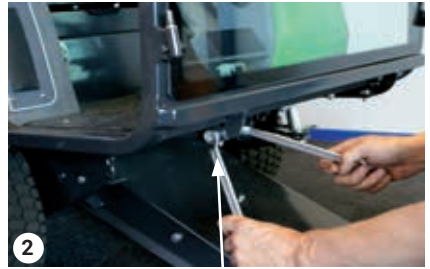
Bolts under base plate
