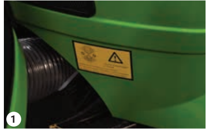
1 Articulation joint warning
