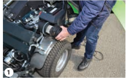
Air filter housing / Filter element
