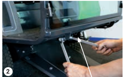
Bolts under base plate
