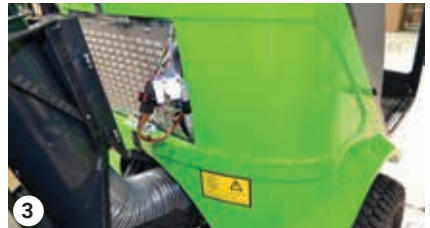
3 connectors behind grate
