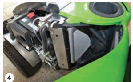
Clean coolers using compressed air
