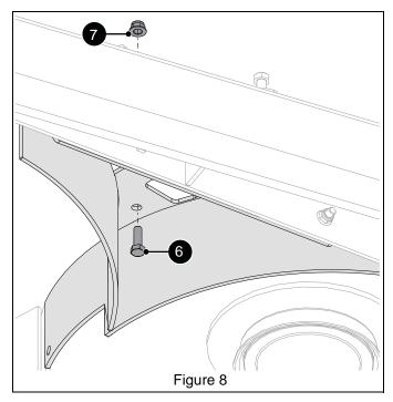
6. Secure discharge baffle (item 3) to deck with two 5/16" nyloc flange nuts. See Figure 9.
