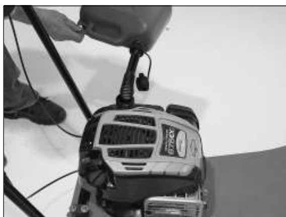
2) Hold the canister as shown in the image. Only ever pour in a small quantity at a time and monitor the fill level.
