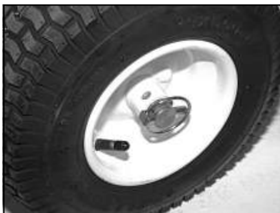
1. Engage the steerable freewheel: Insert the linchpin through the axle only.
