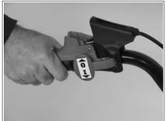
4) Operating the gear lever switches on the brush drive.
