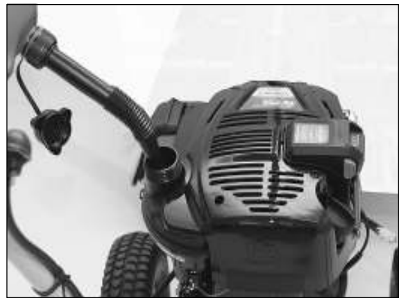
2) Hold the canister as shown in the image. Only ever pour in a small quantity at a time and monitor the fill level.
