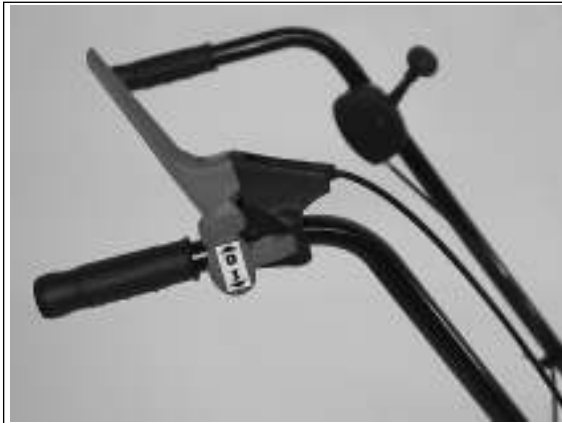
1) The gear lever for the sweeper brush drive is located on the handlebar.
